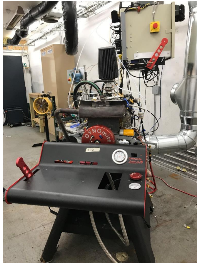
Figure 3.2: Engine setup showing 9" water brake dynamometer
